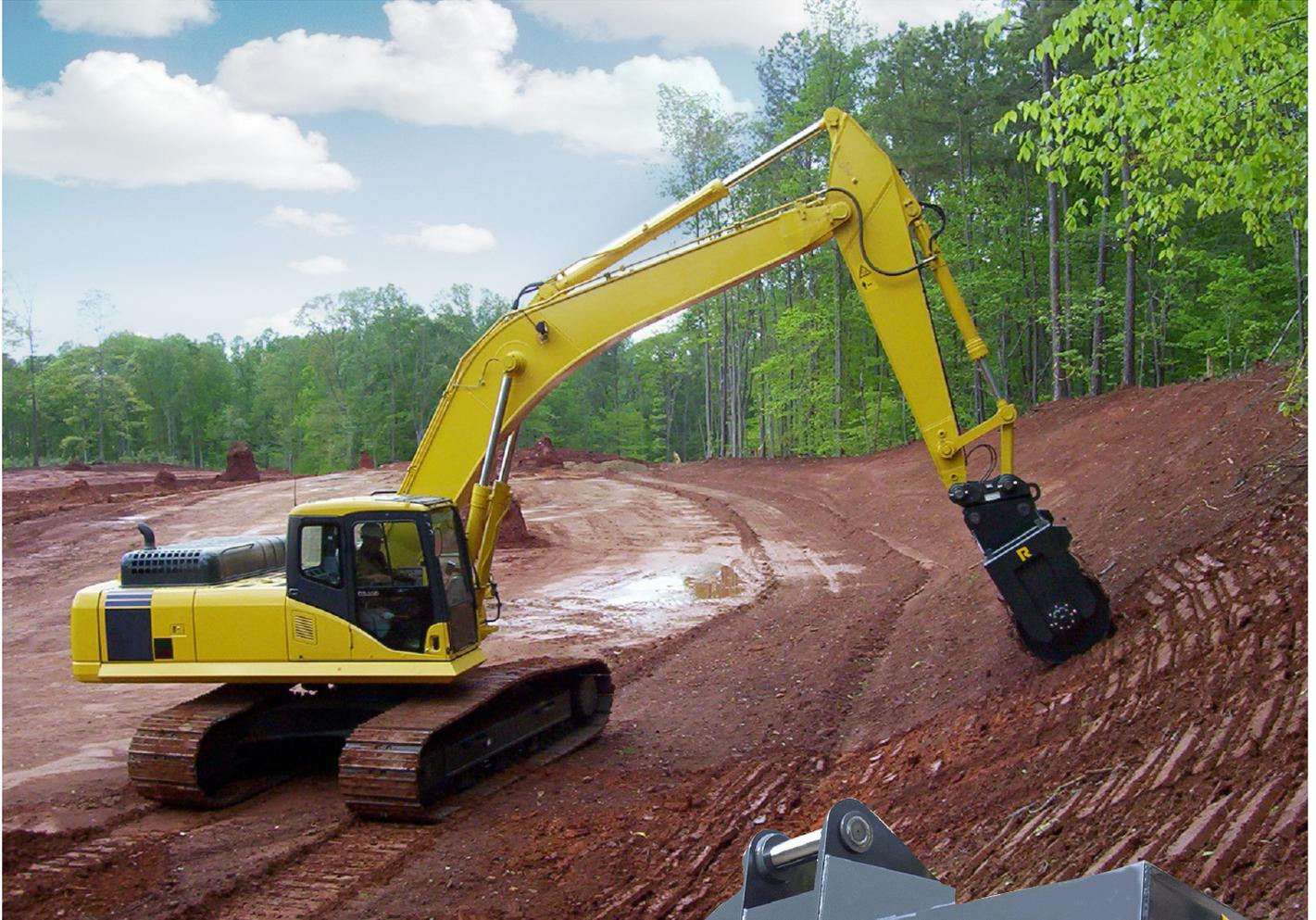
**P**ark your dozer and pack slopes eight to ten times faster. Plus with the Thompson Slope Packer® you can pack in tight clearance areas eliminating damage to silt fences, trees, and culverts.
